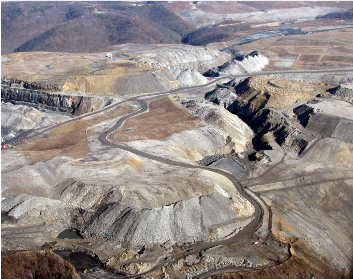
Figure 2. Oblique aerial photograph of large MTR operation near Kayford, West Virginia. Photo courtesy Vivian Stockman/OVEC.
